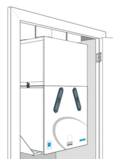
Typical cupboard installation of MRXBOXAB-ECO3B
